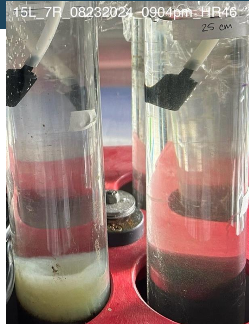
Alum dosed (left) and untreated (right) cores in low oxygen + high pH conditions.
